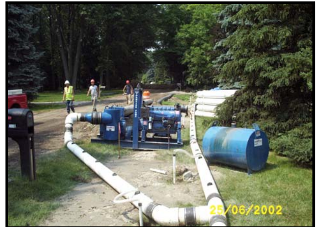
Thompson Pump's Rotary Wellpoint Pump has high air handling capability and is capable of dewatering systems 1,400' long
