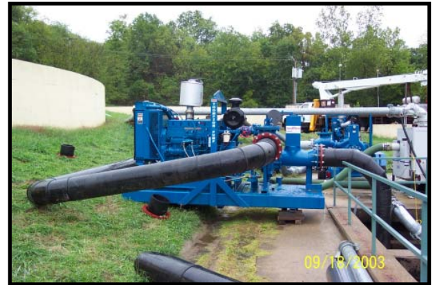
The 6-inch and 12-inch Solids Handling Compressor-Assisted High Pressure Thompson Pump with ENVIROPRIME ® Priming System .
