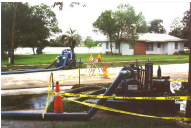
Above: Two Thompson Pumps working to move flood water in a residential area to a near-by lake. Right: Floodwater softened the ground enough to sink this mini-van up to the axles and floorboards.
