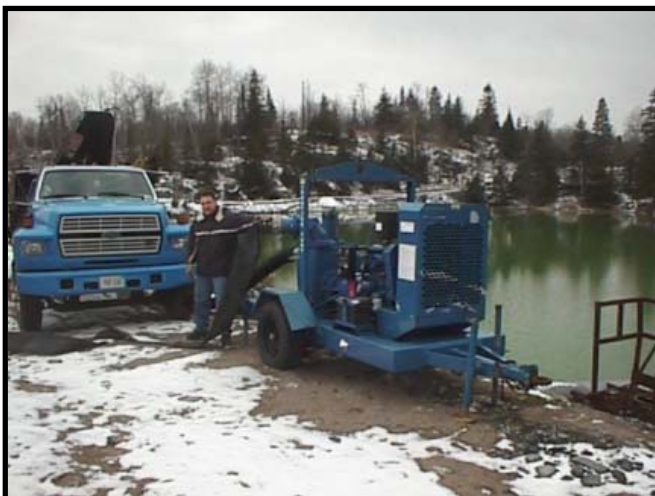
Sam Scola, INCO Limited, Sudbury Operations stands by his Thompson 6-inch Compressor-Assisted Dry-Prime Pump.
